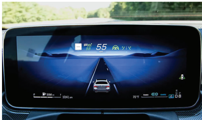
With the active driving assistance system engaged in the 2022 Mercedes-Benz C-Class, the driver’s instrument panel shows the car within the lane lines, while the green steering wheel with hands icon indicates that lane centering assistance is functioning. Photo: John Powers/Consumer Reports
